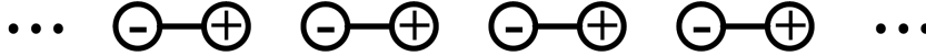
Figure 7.1: As a series of dipoles line up end to end, one can see a current flowing through the line of dipoles as they oscillate back and forth in their polarity. This is similar to how displacement current flows through a series of capacitors.
